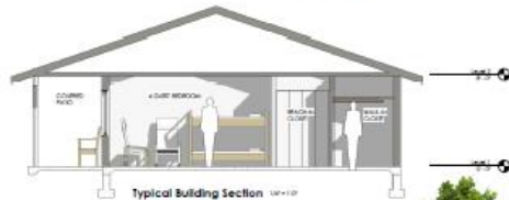
Typical Building Section 1/4"=1'-0"
